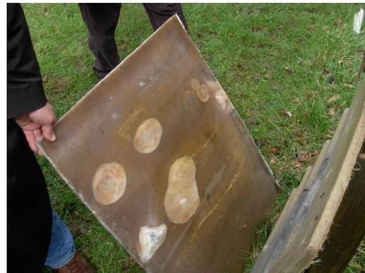
The lower left corner of the photo shows the panel shot by a 12 gage shot gun with number 4 shot. This was repeated nine times. The panel was shot from a distances of 15 feet. The upper left corner of photo reflects three hits from a 38-caliber revolver. The distance to the panel was 10 feet. The upper right center of the photo shows five shots from a 357 magnum at 15 feet. The photo of the rear of the panel shows no penetration by any of the shells or pellets.
